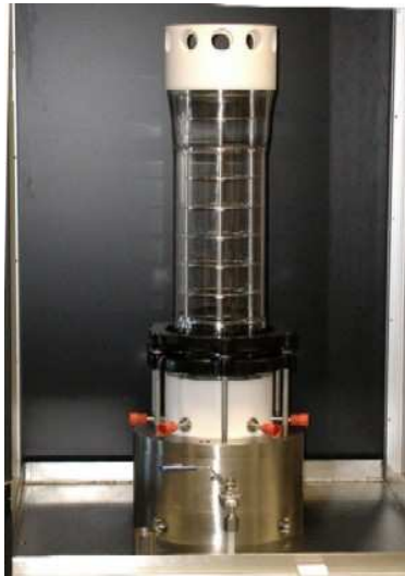
Figure 9. Standard design includes an oscillator base and a reactor tube top section.
