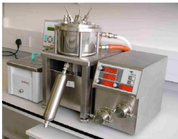
Figure 3. This small Spinning Disk Reactor can serve as a complete mini-development plant.
