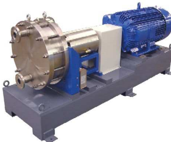
Figure 5. Purposely generated cavitation enhances mass transfer and produces uniform heating.
