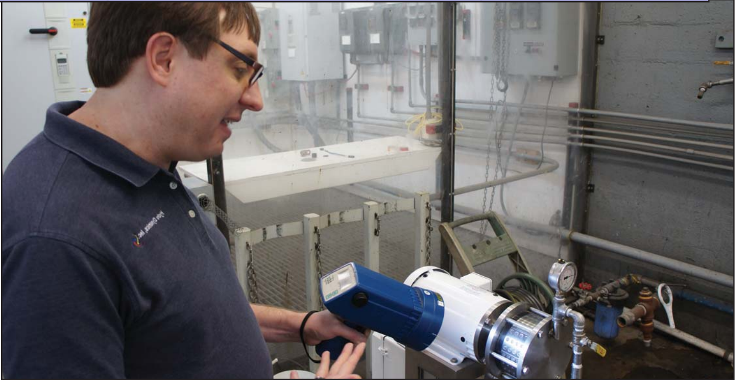
Dr. Doug Mancosky, Vice President of Research and Development at Hydro Dynamics, Inc. uses a strobe light to show the cavitation in the ShockWave Power Reactor.
