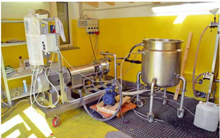
SPR pilot reactor in the set up used to perform controlled cavitation tests.
