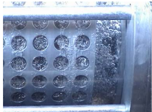
Figure 1: A small ShockWave Power™ Generator during gas / liquid mixing with a clear housing for ease of viewing.
