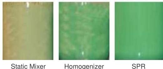
**Mixing of Shear Sensitive Compounds:** The SPR can be configured for low shear mixing. This allows for the treatment of shear sensitive compounds such as proteins, polymers, and citrus pulp without damage.
