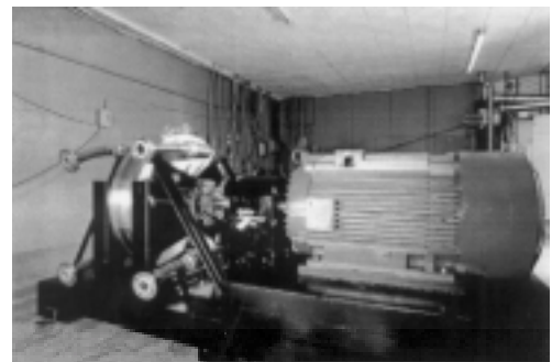
Figure 2: A commercial size ShockWave Power™ Generator complete with electric motor.
